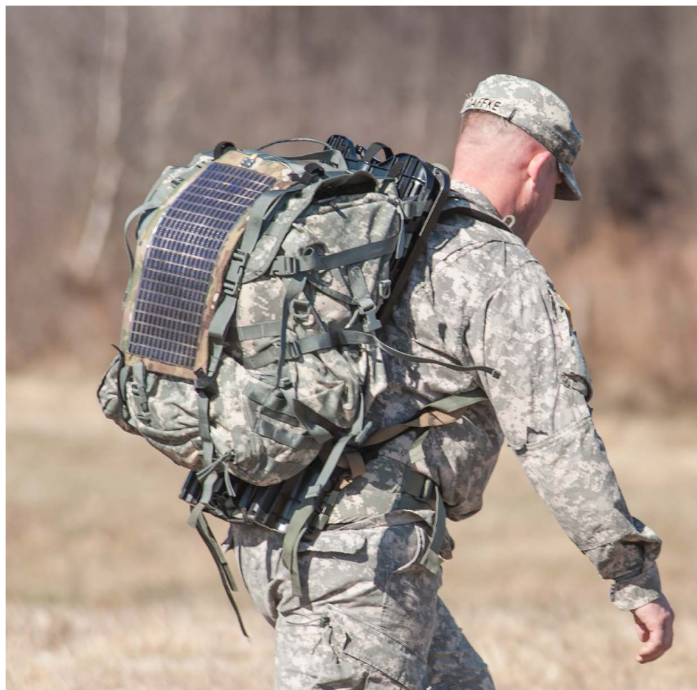
A soldier conducts dismounted maneuvers wearing a photovoltaic solar panel harvester during an energy-harvesting technology demonstration. (Photo: David Kamm, NSRDEC)
