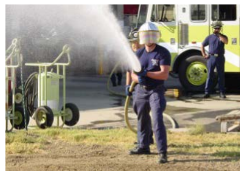
NoFoam System Nozzle Discharge Check at NAS Lemoore (Source: Kudo, Rance. TR-2329-ENV NoFoam System for Automotive Fire Apparatus Vehicle Foam Discharge Check. April 2010.)
