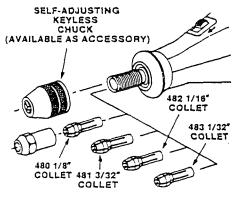
sizes, are available for your Moto-Tool. To install a different collet, remove the collet nut and remove the old collet. Insert the unslotted end of the collet in the hole in the end of the tool shaft. Replace collet nut on the shaft. Always use the collet which matches the shank size of the accessory you plan to use. Never force a larger diameter shank into a collet.
