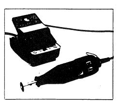
If you need it, single-speed models also can have speed control by the addition of a foot control unit.
