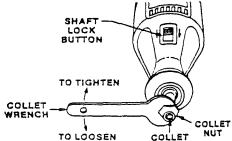
**COLLET** — Consists of a collet nut and collet. To loosen, first slide shaft lock forward and rotate the shaft by hand until the lock engages the shaft preventing further rotation.
