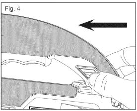
top handle snaps and locks into place (Fig 4). Release the handle release buttons.
