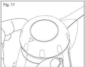
**IMPORTANT:** When you are manually scroll cutting always hold the saw handle in one hand and rotate the scrolling knob with your other hand, while applying pressure to the front of the saw so it does not jump out of the workpiece.
