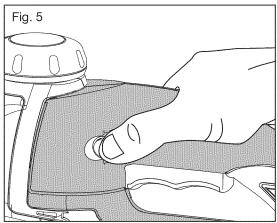
4. To lock the on/off trigger switch in the "on" position, press trigger switch and while holding it "on", press in the lock-on button from either side. The power lock-on button allows the operator to keep the jig saw running without squeezing the trigger switch. This feature is convenient for continuous sawing applications.
